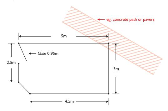
• If there is any soil to be retained (up to a maximum depth of 600mm), mark this into your plan with the symbol shown below – include the approx soil depth.
