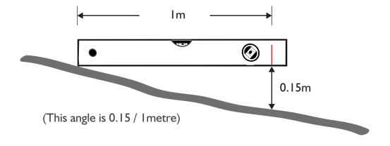
• Draw the ground slope in each elevation box provided on our site measure form. Show and dimension any irregularities in the ground, including flat spots or hollows and mark the angle of the slope as below.
